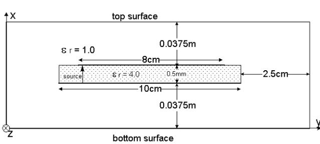
Figure 3 two-plane test structure
