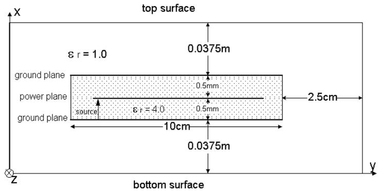
Figure 5 three-plane test structure
