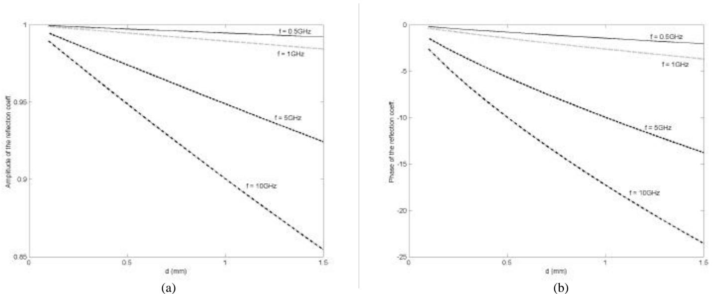
Figure 2. Reflection coefficient at the open end of two parallel planes (a) amplitude (b) phase
