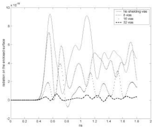
Figure 7. Radiation from the board with shielding vias
