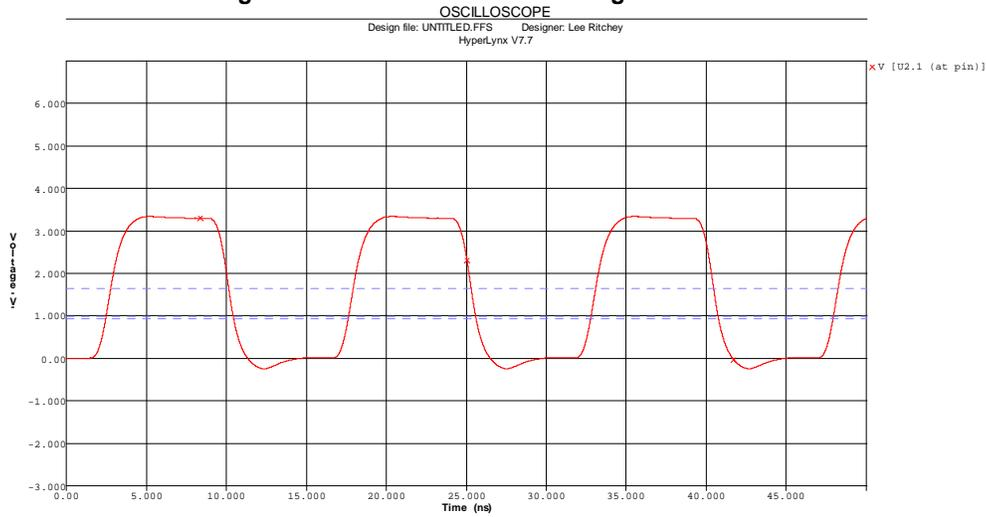
**Figure 3. PCI Bus Waveform Driving a 65 Ohm Line**
