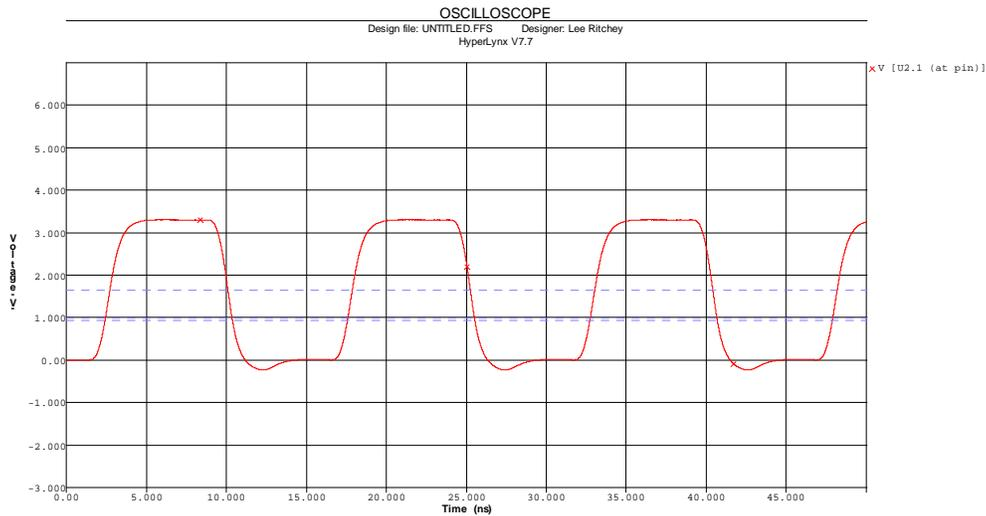
**Figure 2. PCI Bus Waveform Driving 50 Ohm Line**
