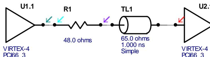
Figure 1. PCI Signal Driving a Six Inch Long Transmission Line
