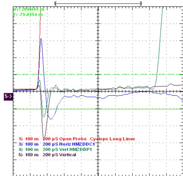
**Figure 4. Impedance vs. Length Over 3313 Glass**
