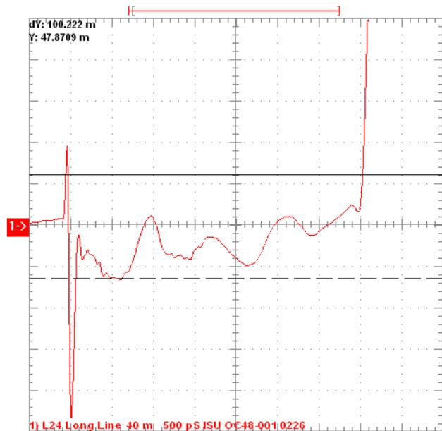
**Figure 2. Impedance vs. Length Over 1080 Glass**
